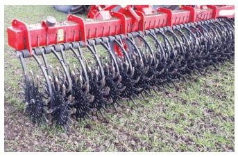
The rotors are off-setted and arranged in a staggered position to better pass the plant residues and avoid any blockage by the stones. Their spacing of 87 mm guarantees uniform peeling over the entire width.
