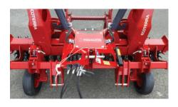
Standard: depth control wheels with manual offset and height adjustment by rack and sprocket. Manual lock actuated from tractor cabin with rope.
