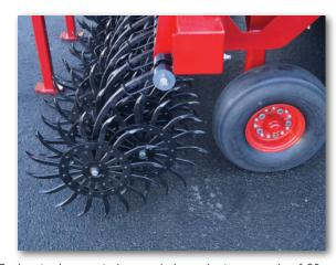
Each rotor is mounted on an independent arm made of 26 mm cast steel itself articulated on a 30 mm shaft and damped by a spring that exerts significant pressure; this arrangement allows a rotor to overcome an obstacle without disturbing the neighbouring rotors and to adapt to the unevenness of the ground.
